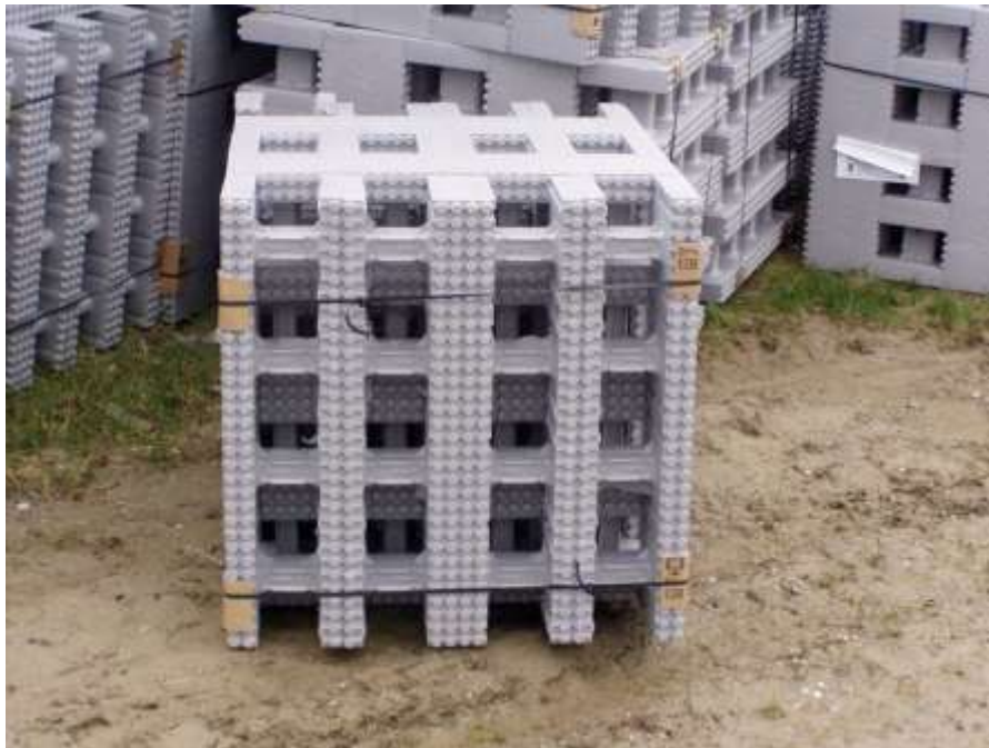
Tying, corner protecting
